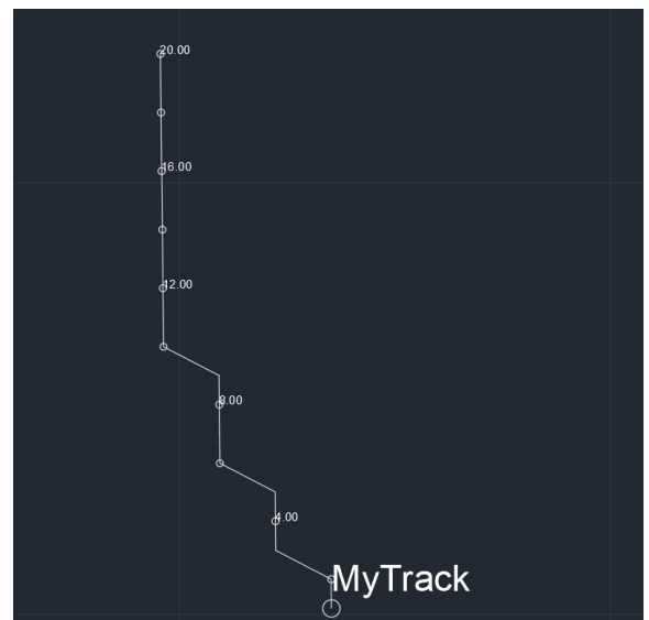
Figure 14.1 Examples of a track plotted by gMapIoAcadPLDraw (an AutoCAD script execution result)
